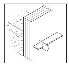
**AR Quick Strip Tys** are available for wall thicknesses ranging from 100 mm to 750 mm (4" to 30") and are designed to reduce waler and bracing requirements.
