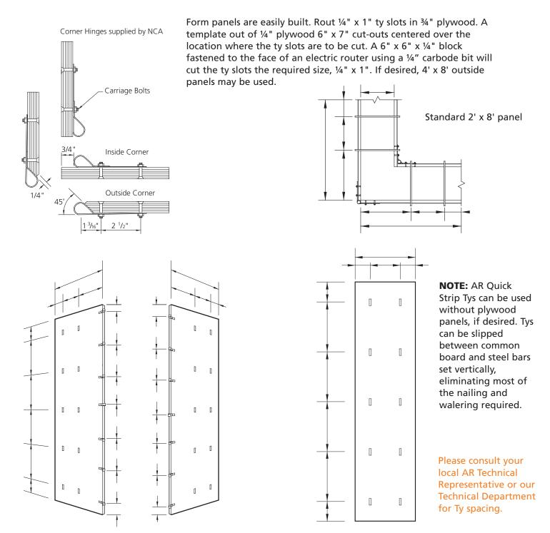
Corners are made from <sup>3</sup>/<sub>4</sub>" plywood, and hinges supplied by AR. Corner shown is the standard 2' and works best on most jobs. Corners are connected by inserting a <sup>5</sup>/<sub>8</sub>" rod through the hinges.
